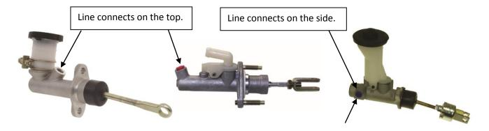
Note: Master cylinders that have the pressure connection at the bottom of the master cylinder are not a good candidate for this procedure. Starting with the system completely connected, reservoir full and if possible a length of tubing attached to the bleed screw directed into a waste fluid container:
