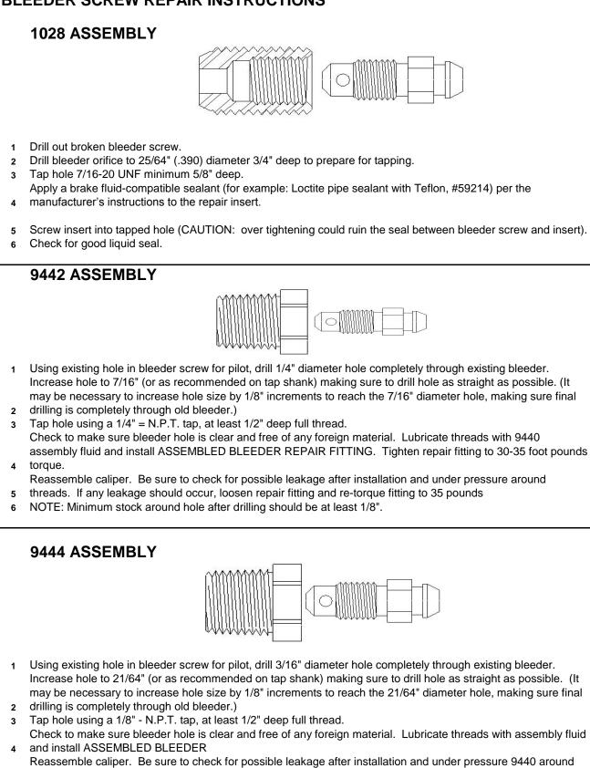
Reassemble caliper. Be sure to check for possible leakage after installation and under pressure 9440 around threads. If any leakage should occur, loosen repair fitting and re-torque fitting to 35 pounds. fitting and retorque fitting to 35 pounds.
