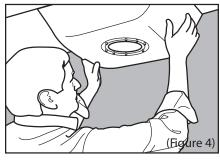
Inspect fuel tank for rust and physical damage. Repair or replace if signs of either. (Figure 4) Allow tank to sit for half hour or until completely dry.
